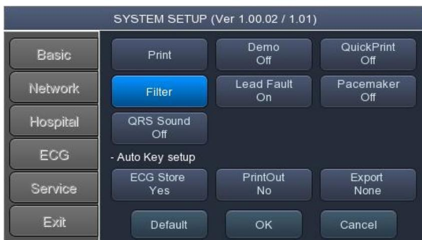
Upon selection, the Filter Setup menu, shown below, will appear. Use either the rotary key or touch screen to navigate and select menu items to edit. After editing, OK must be selected in order to apply the changed value.
