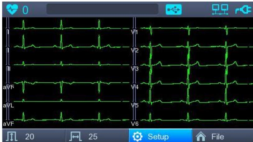
Choose the 'Setup' button on the initial ECG main screen to change preferences.
