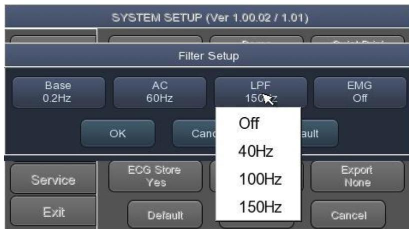
Select 'ON' when applying 'EMG' filter; otherwise, select 'OFF.' Setup values will be shown on the bottom of the printout form as 'EMG:On' or 'EMG:Off' when applying the filter.
