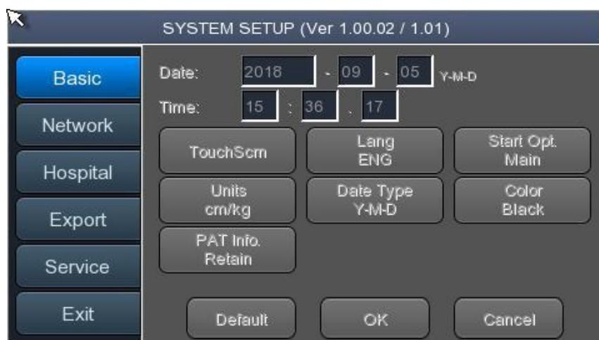
'PAT Info.' menu is to set up whether the patient information is retained or not, when you move the main screen of the ECG. When you click the menu, 'Retain' will be set up and when clicking the menu again, 'Delete' will be set up. Default is set as 'Delete'.
