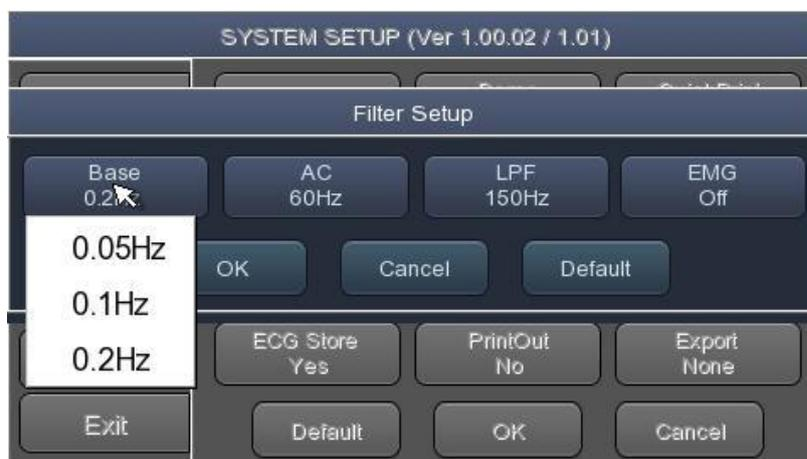
There are three types of an AC power noise filter; 60Hz, 50Hz and OFF. When set to OFF, the filter will not be applied. If the filter is set to 50Hz or 60Hz, then the AC filter will remove 50Hz or 60Hz power noise correspondingly. In the U.S., the AC filter should be set to 60Hz. Check the properties of your power source before setting AC filter properties.
