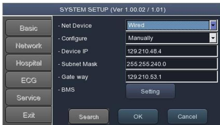
The mode of network connection can be selected as Wired or Wireless in 'Net Device' setup.
