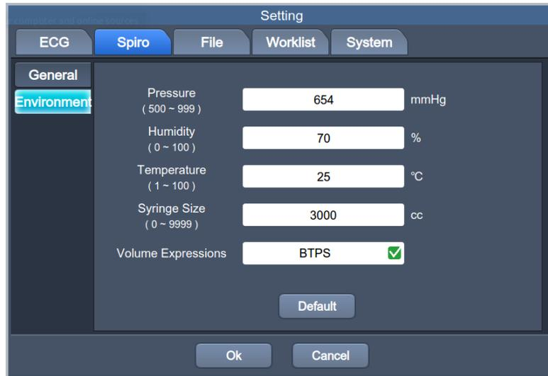
The screenshot shows a 'Setting' dialog box with tabs for ECG, Spiro, File, Worklist, and System. The 'Spiro' tab is active, and the 'Environment' sub-tab is selected. The settings are as follows:
