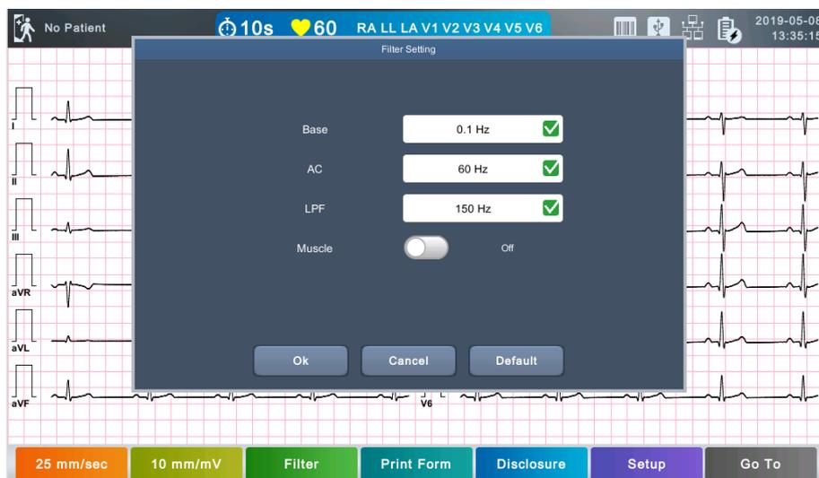
The ECG signal may contain not only ECG data, but also power noise, baseline drift by breathing, and EMG signals. Therefore, proper use of the filter when the signal is bad can give you a good ECG signal.
