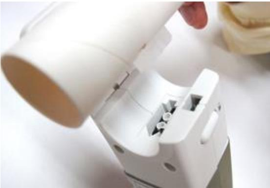
(2) Put the mouthpiece on the inserting lot made on the open side.
