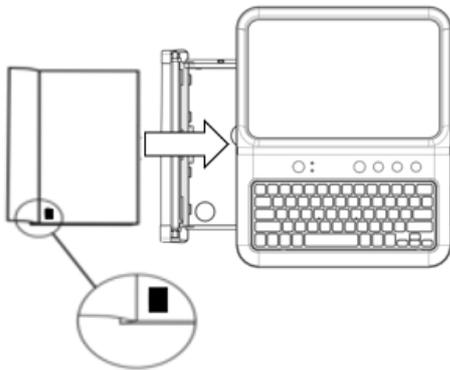
Insert the ECG recording paper with the area to be printed facing up as shown in the picture, making sure that the black mark on the paper is located at the bottom.
