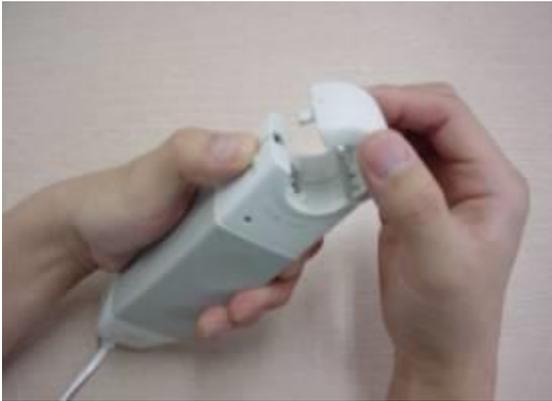
(1) Press the Front Cover Lock Switch on the top left corner of spirometer handle and open the Front Cover in semi-circle shape.
