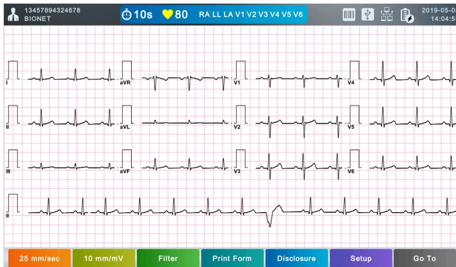
The background color of the screen output of the ECG waveform can be white or black, which you can change in the Setup → ECG → General → Background menu.
