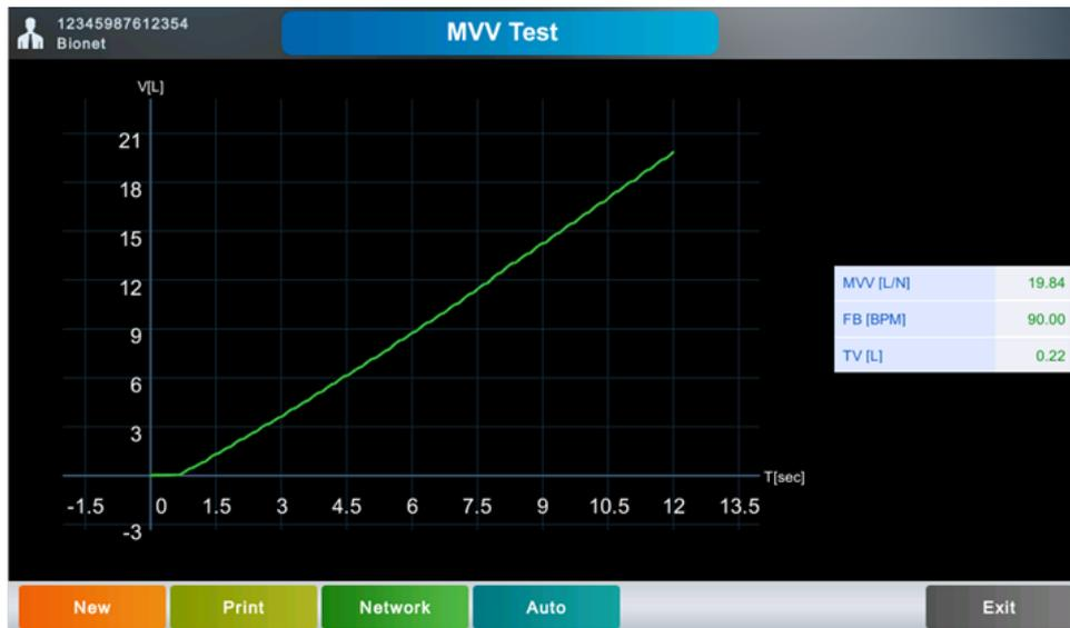
When the set time (TMVV) - 12 seconds - passes, the test ends and the result is displayed on the screen. MVV, respiratory cycle (FB), and total respiratory capacity (TV) are calculated and displayed at the top of the screen. Touch [Stop] to finish during the test. You are moved to the initial MVV test screen.
