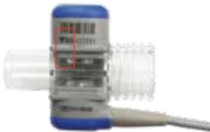
There is an arrow on the airway adapter and a matching arrow on the CAPNOSTAT® 5. These need to be pointing toward each other when you install the airway adapter.
