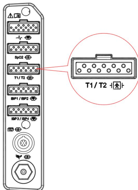
Temperature Measurement Sensor and Cable
