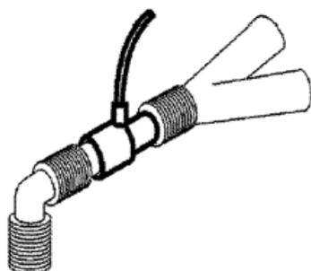
For intubated patients with an integrated airway adapter in the breathing circuit: Connect the male luer connector on the straight sample line to the female port on the airway adapter.
