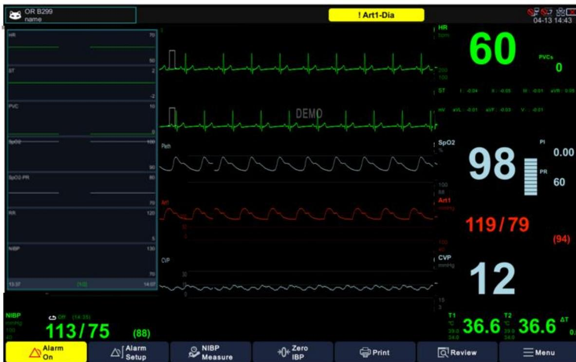
You can continue to monitor the main screen waveform and parameter box while watching the trend data for up to 7 parameters for up to 6 hours. The pop-up trend graph follows the display order indicated by each parameter in the trend setup and is updated with new trend data every 60 seconds.
