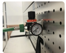
DISS male inlet port with pressure regulator
